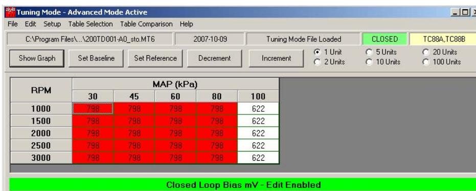
Further, by mapping the AFR cells to A/F ratio of 14.6 in the “milder drive ranges” the ECU will run in closed-loop (red cells) for those ranges (now at a lower A/F of approx 14.1 due to the bias table adjustment). At high load and WOT the cells are mapped to a lower and richer A/F ratio forcing the ECU to run in open-loop mode (white cells).
