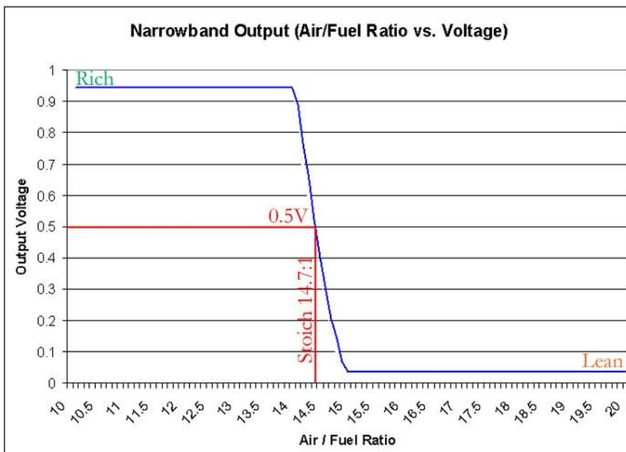
However, stoichiometry at A/F 14.7 does produce the hottest combustion and the hottest Exhaust Gas Temperature (EGT). Thus there have been complaints that the 2007/2008 Harleys run excessively hot, in particular at idle. The EGT drops at either side of stoichiometry (A/F 14.7). A richer A/F ratio at say 13.5 produces less heat and gives maximum power/torque (but less perfect combustion, and more emissions).
