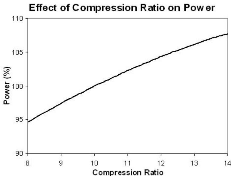
Note. In the days of Volkswagen-trike engine tuning it was popular to increase the reliable air-cooled low-compression ratio VW engine to high compression ratio in order to increase power. Due to lack of sufficient air cooling (air cooling system usually dismantled) engine overheat and breakdowns was common. Reducing compression ratios back to 8.5:1 usually cured overheating problems.
